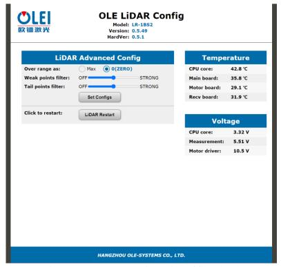
Figure 10 Parameter configuration of filter level
