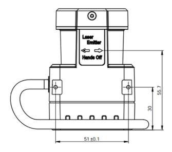
Figure 1: Back mounting interface of LR-1BS1
