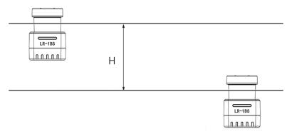
Figure 22 Placement of two LiDARs with parallel offset
