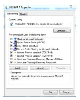
Figure 6: Step 2 of computer IP setting
