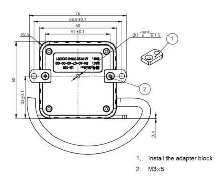
Figure 2: Bottom mounting interface of LR-1BS1
