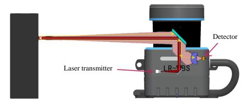
Figure 8 Diagram of LR-1BS1 LiDAR work principle
