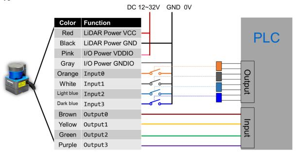
Figure 13 Typical electrical connection
