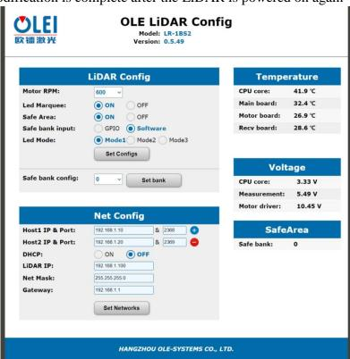
Figure 9 Parameter configuration of web page
