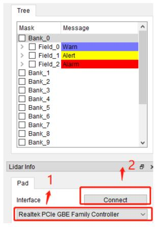
Figure 18 Connecting the LiDAR
