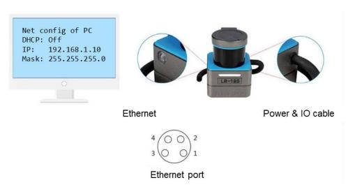
Figure 3 Diagram of electrical interface
