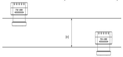
Figure 24 Placement of two LiDARs upside down, parallel offset
