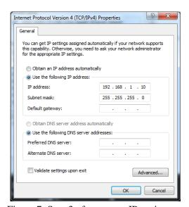
Figure 7: Step 3 of computer IP setting
